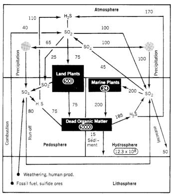
The circulation pattern of sulfur in nature and estimated fluxes. Circled numbers are amounts present in different reservoirs; other numbers are yearly fluxes, all in million tons sulfur units
